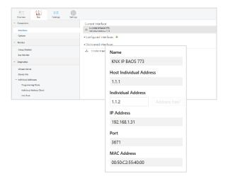
The individual KNX device address and the individual KNX addresses for additional tunneling connections can be changed within the ETS project, after the device has been added to the project.
