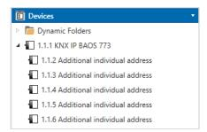
Each individual KNX address can be changed by clicking on the list entry and typing in the desired address into the "Individual Address" text-field. If the text-field frame switches to color red after entering the address, the address is already taken within your ETS project.
